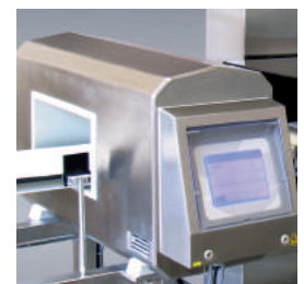
Tunnel metal detector
