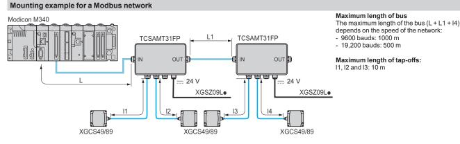
Examples of connection to a Schneider Electric automation platform **Direct connection** Connection via a TWDXCAISO isolation box
