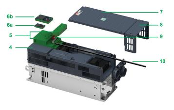
Another form of ATV340 with VW3A1111 (advanced keypad), and VW3A3800 (Hoist option), and connector under front cover and conduit box
