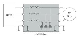
Altivar machine drive with dv/dt filter
