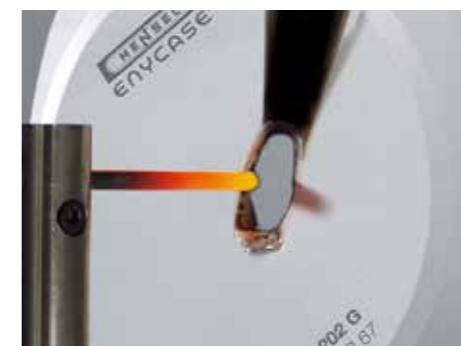
Burning behaviour: glow wire test according to IEC 60695-2-11: up to 960 °C, flame-retardant, elf-extinguishing
