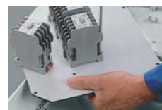
Device installation on mounting plates
