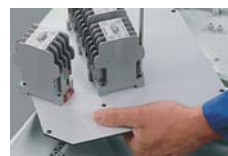
Device installation on mounting plates
