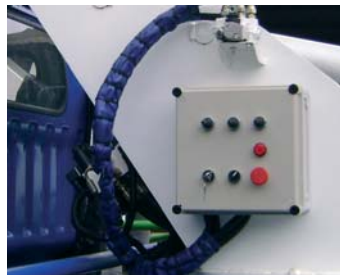
Enclosure with START-STOP button on a mobile and stationary vehicle.
