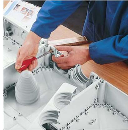
Adjust stepped grommet on the cable diameter.
