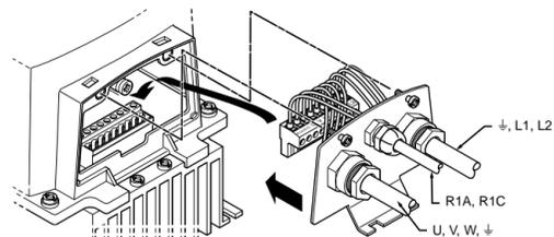
For EMC mounting, radiated emissions EN 55022 class B:
